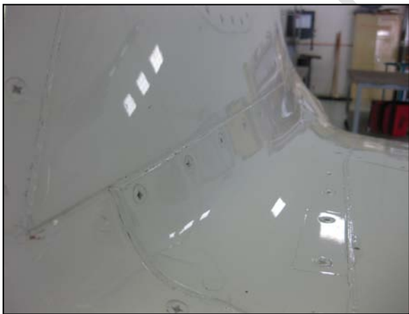
Area of slight cracking and touch-ups
